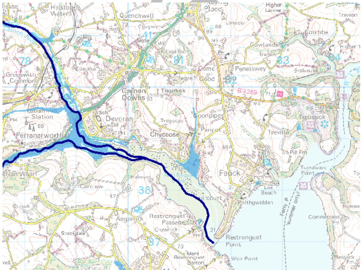
Figure 42: Flood Risk map for Feock Parish – areas identified in light blue are areas at risk from flooding and dark blue are rivers/watercourses. Source: Environment Agency interactive online map.
