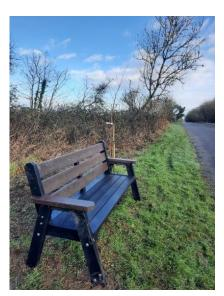
The benches are made out of 100% recycled mixed waste plastics and we have two more benches still to install over the next couple of months.
